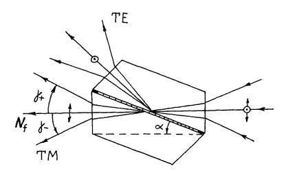
FIGURE 1 Schematic representation of linear prism liquid crystal polarizer. The heavy glass prisms are separated by teflon spacers. NLC layer has a homeotropic orientation.
